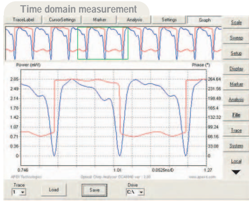
10Gb/s DPSK modulation (phase in red and intensity in blue)
