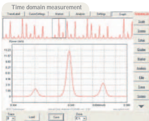
Mode locked fiber laser pulse measurement (4ps pulsewidth)
